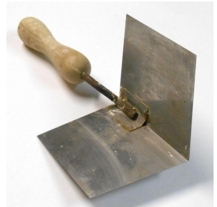
Figure 8-25 Inside Plastering Corner Tool (not an inside Drywall Tool). Corner tool pressure seals and seats the wet cement
