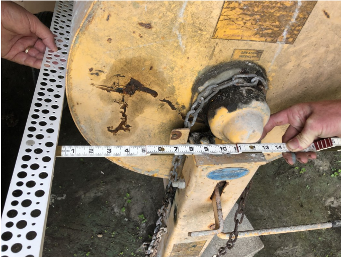
Figure 6B - Measure Radius in inches ( 12 Inches on this mixer - Casing Stop used to aid in measuring)
